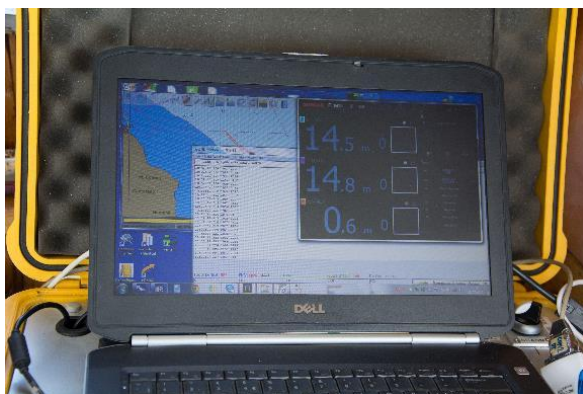
Figure 7.24. Gear monitoring system from Simrad. The screen shows the horizontal net opening of the two nets and the vertical net opening of the net with selector.
