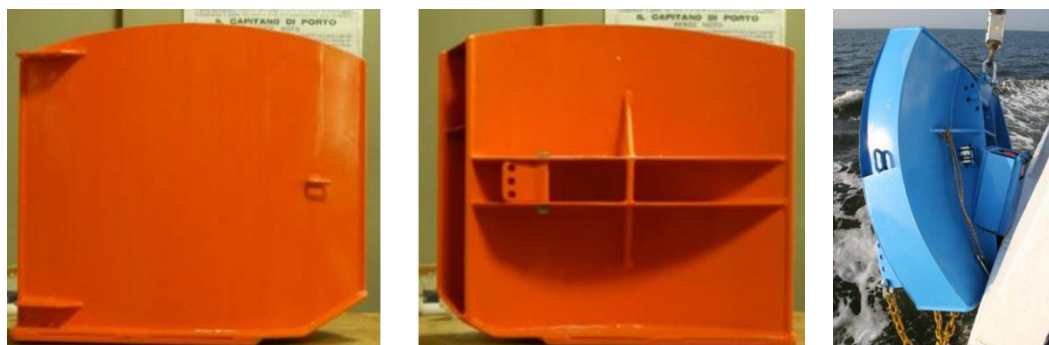
Figure 7.18. Mori Biplan. On the left, the model tested in wind tunnel and flume tank; on the right the full-scale otterboard used during the sea trials.
