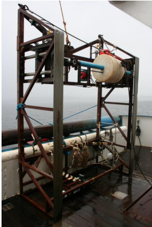
Figure 1.2. The towed sled used to tow the range of cylindrical objects supported on an axle.
