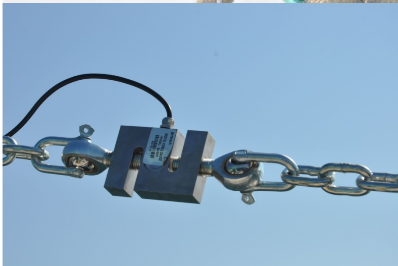
Figure: equipment to measure the fuel consumption and the resistance of the seafloor to trawling
