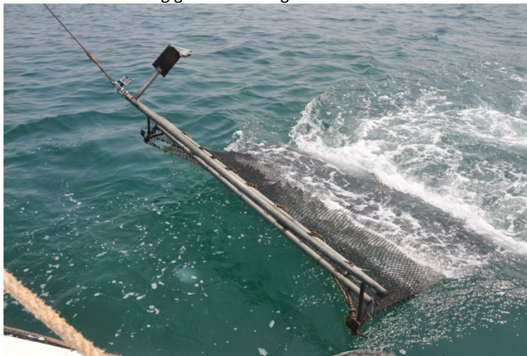
The innovative fishing gear without the steel rope
