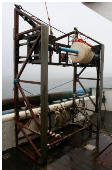
Figure 29. The towed sledge used to tow the range of cylindrical objects supported on an axle.
