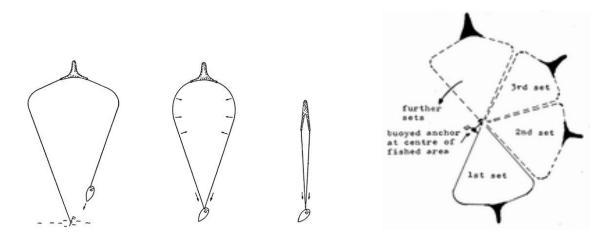
Figure 5. Left: Illustration of three steps in an individual anchored seine haul, Right: the combined gear footprint of a series of four seine hauls (illustration from <u>http://www.fao.org/fishery/geartype/203/en)</u> The direct sea bed impact from demersal otter trawls and the other major towed gears can be assessed from two parameters for each of the major gear components described above: a) the width of the
