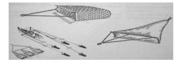
Figure 4. Two different dredge types, with and without with shearing edge, and towed in different ways and numbers (drawing from FAO Fisheries Technical Paper No. 419)
