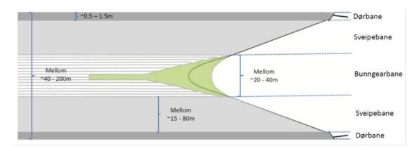
Figure 2. Conceptual footprint from standard otter trawls with three types of sea bed impacts: 1) the track affected by the otter boards ("Dørbane"), 2) the track influenced by the sweeps ("Sveipbane") and 3) the track affected by the trawl itself ("Bunngearbane"). Illustration from Buhl-Mortensen et al. 2013.
