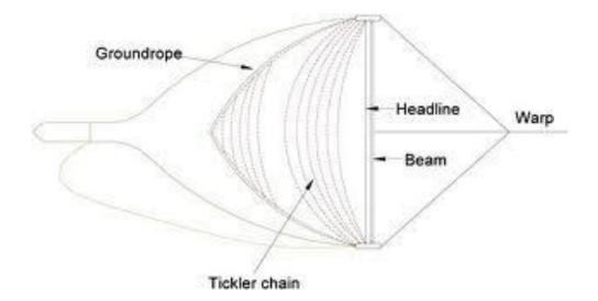
Figure 3. Drawing of beam trawl with warp, beam, shoes, tickler chains and ground gear (illustration from FAO Fisheries Technical Paper 472)
