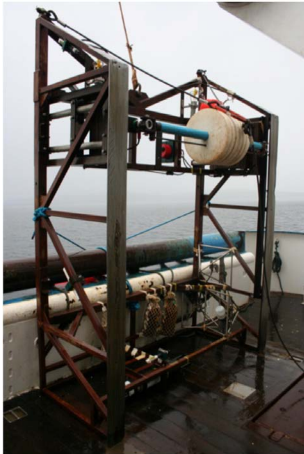
Figure 2. The towed sledge used to tow the range of gear components.
