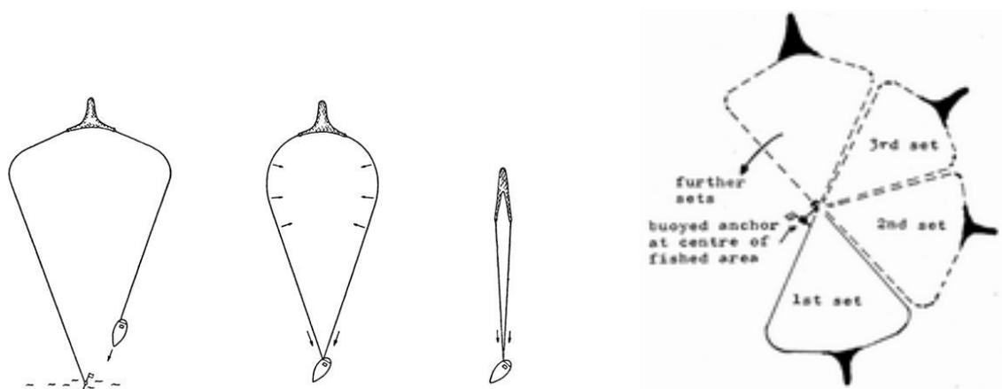
Figure 5. Left: Illustration of three steps in an individual anchored seine haul, Right: the combined gear footprint of a series of four seine hauls (illustration from <http://www.fao.org/fishery/geartype/203/en>) The direct sea bed impact from demersal otter trawls and the other major towed gears can be assessed from two parameters for each of the major gear components described above: a) the width of the
