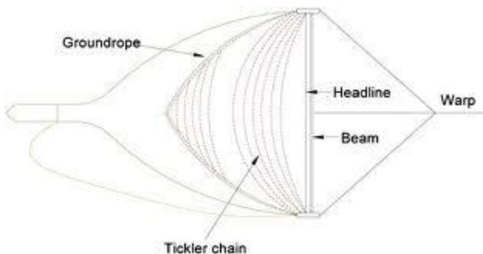
Figure 3. Drawing of beam trawl with warp, beam, shoes, tickler chains and ground gear (illustration from FAO Fisheries Technical Paper 472)
