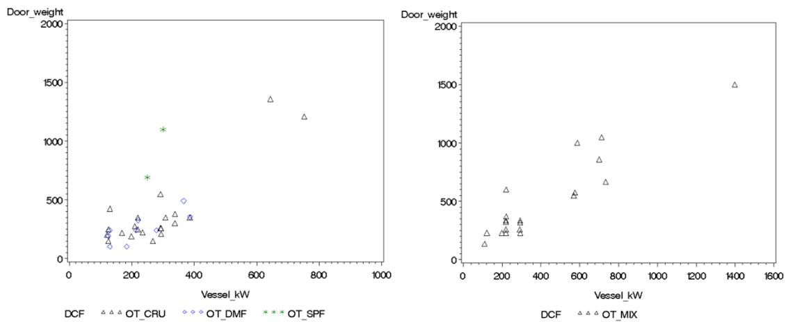
Figure 10. Otterboard (door) weight against vessel kW by metier (OT=Otter board trawls, CRU=crustaceans, DMF=demersal fish, MIX=mixed crustaceans and demersal fish, SPF=small pelagic fish).
