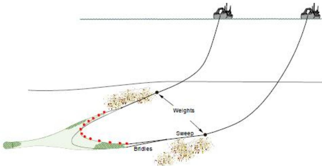
**Figure 4.4.** Pair trawling with a bottom trawl. (Illustration from Buhl-Mortensen et al. 2013).
