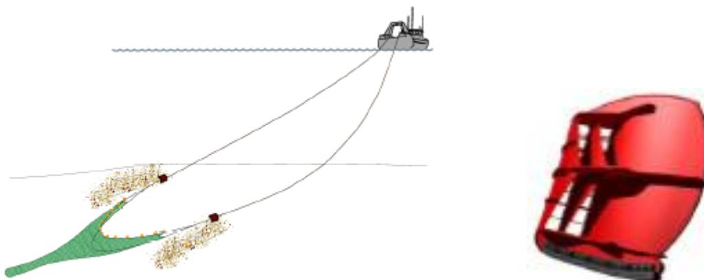
**Figure 4.1.** Left: illustration of bottom trawling using a single trawl and right: typical bottom trawl door (Illustration from Buhl-Mortensen et al. 2013).
