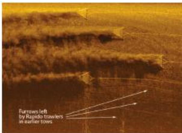
**Figure 5.6.** Resuspension of sediments caused by Rapido beam trawling in the Adriatic Sea. Evidence of the furrows left by Rapido trawlers in earlier tows can be seen in the lower part (image from Luchetti and Sala 2012)
