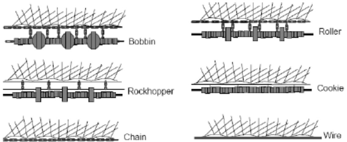
**Figure 4.2.** Examples of ground gear designs for bottom trawling. (Illustration from Buhl-Mortensen et al. 2013).
