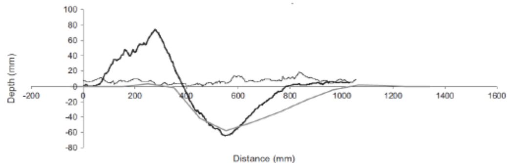
**Figure 5.4.** Laser readings before (dotted line) and after (solid black line) contact with a trawl door in muddy sand, compared with the predictions of a classic FE model of plasticity (solid grey line) (from O'Neill et al. 2010).
