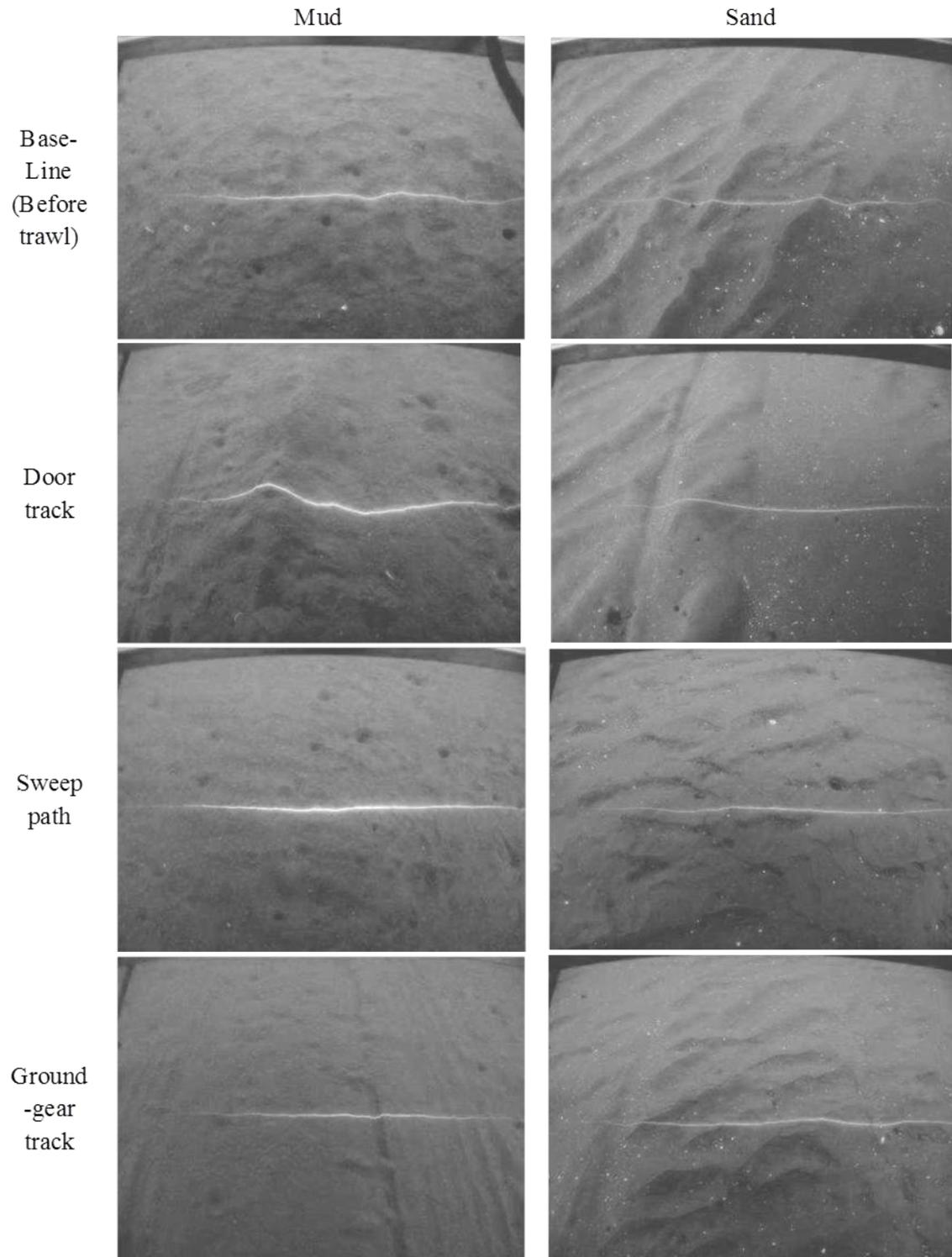
**Figure 5.3.** Photos of sediments before and after contact with various components of the trawl in mud and sand. Each photo also shows a laser profile (from DEGREE 2010).
