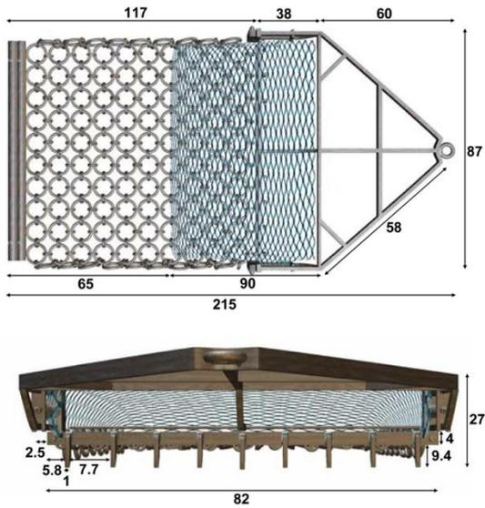
**Figure 5.7.** Front and top view and dimensions (mm) of scallop dredges in use in Scotland (O'Neill et al 2013)
