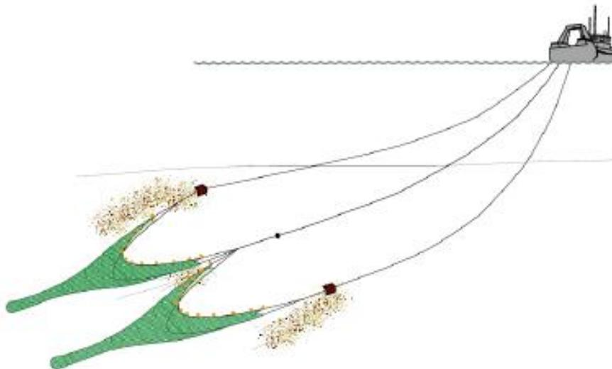
**Figure 4.3.** Bottom trawling using two trawls (twin rig trawling). (Illustration from Buhl-Mortensen et al. 2013).
