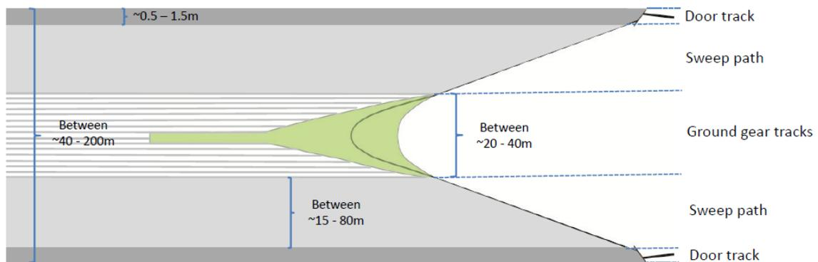
**Figure 5.1.** Conceptual footprint from standard otter trawls with three types of sea bed impacts: 1) the track affected by the otter boards (Door track), 2) the track influenced by the sweeps (Sweep tracks) and 3) the track affected by the trawl/groundgear itself (Ground gear tracks) (Illustration Buhl-Mortensen et al. 2013).
